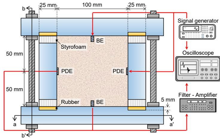
Fig. 1 Schematic drawing of measurement system for elastic waves
